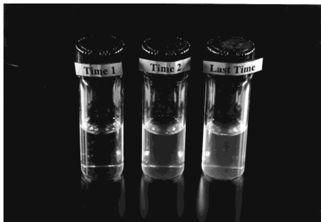
Figure 9—Reconstituted vials of lyophilized bovine IgG in 0.01 M potassium phosphate with 0.22 N NaCl removed during secondary drying, showing development of turbidity in the reconstituted product.
